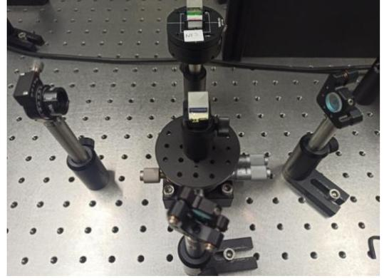
Figure 5 Picture of the Sagnac-Like interferometer
